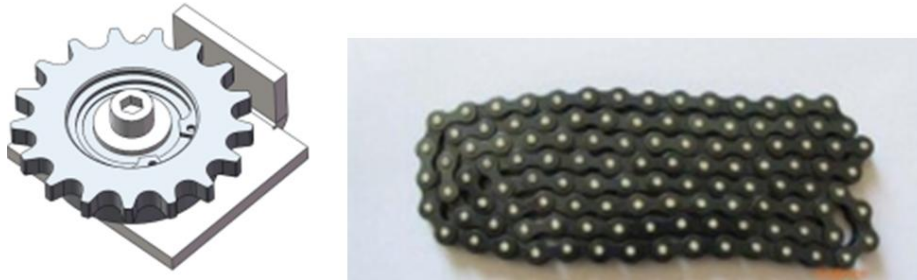
Figure. 4.15 Tension sprocket and chain
