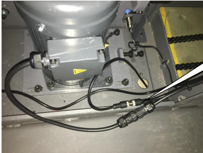
Figure 4.6 Turntable induction wire connection
