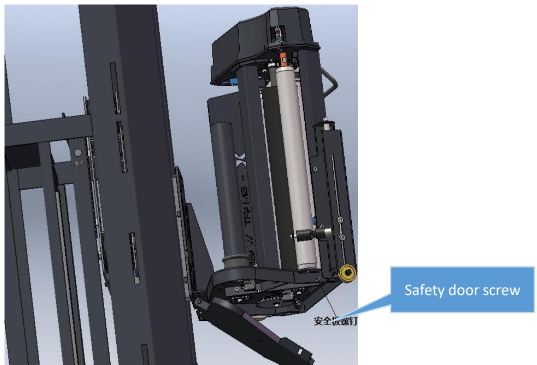
Figure 4.14 Open the bottom safety board
