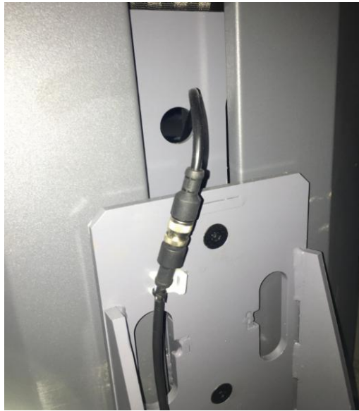
Figure. 4.11 Aerial plug connection of film carriage
