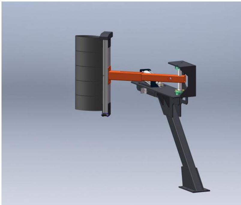
Figure 3.4.1 automatically film cutting and clamping device
