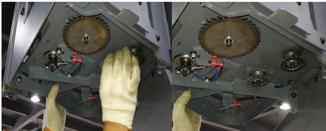
Figure. 4.16 Installation of tensioning sprocket
