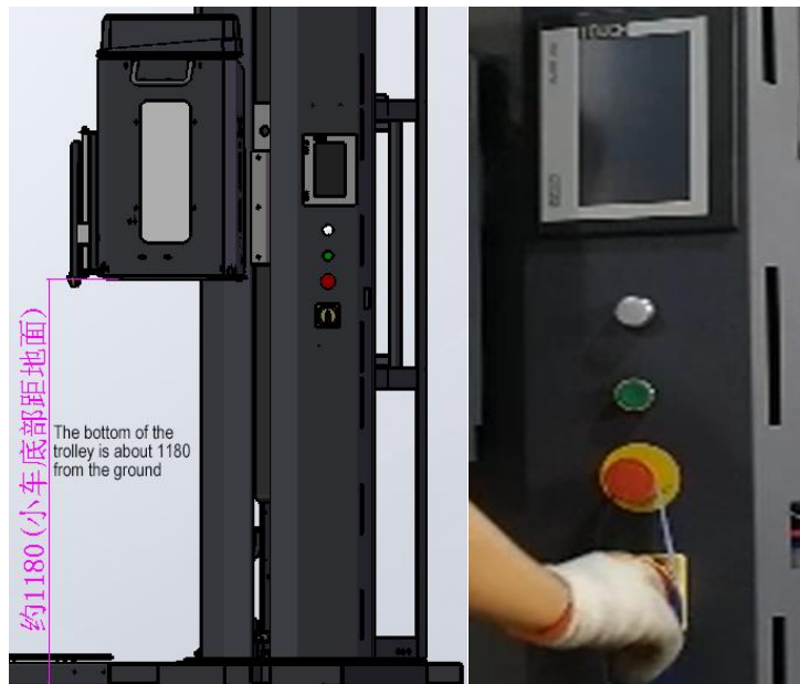
4.12 Turn off the power after the film carriage rises to a suitable height
