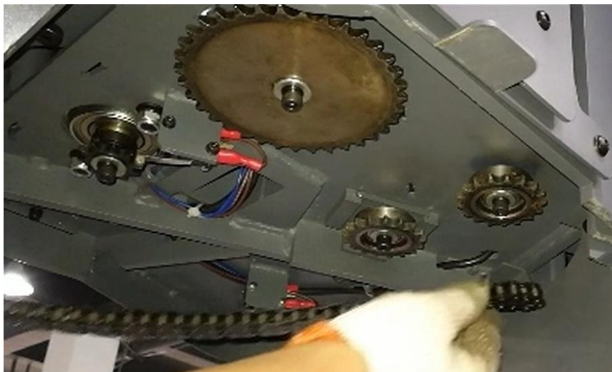
Figure. 4.16 Installation of tensioning sprocket
