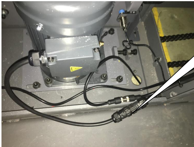
Figure 4.5 Cable connection of turntable motor
